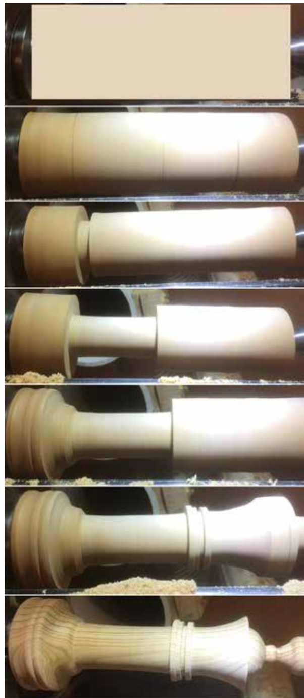
The process of turning a chess piece - in this case, a queen.
